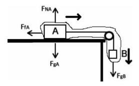
In this example,  $F_{gA}$  and  $F_{NA}$  do not affect the acceleration, so the Net Force is just  $F_{gb}$ – $F_{fA}$ .
