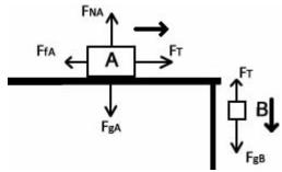
Draw a force diagram for each separate object in the system. Remember the direction each one accelerates is the positive direction.
