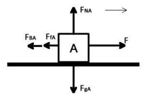
$\Sigma F = ma$   $F - F_{fA} - F_{BA} = m_A a$   $75 - (0.2)(50) - F_{BA} = 5a$   $65 - F_{BA} = 5a$   $65 = F_{BA} + 5a$   $65 - 5a = F_{BA}$
