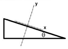
In the example below, I chose downhill to be the positive X direction (because that is the direction the block would accelerate if it does!).
