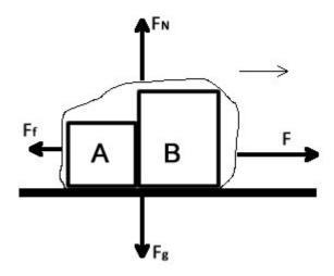
It accelerates to the right, so our Net Force will be Right minus Left. (Note the Normal Force here equals the combined weight of the two blocks.)
